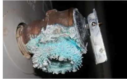
Photo 2 Heavily Corroded Relief Valve
