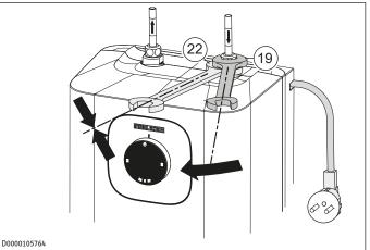
NOTICE: When tightening the fittings, counterhold with a suitable spanner.
