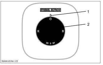
1 Heat-up and index indicator 2 Temperature selector
